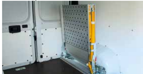
Anti-slip anodised aluminium perforated platform
