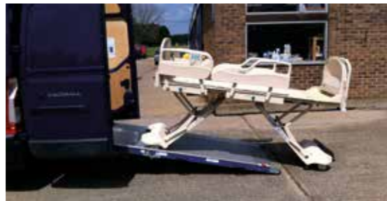
Anti-slip anodised aluminium platform
