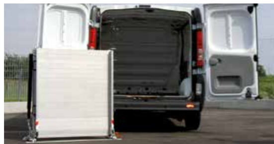
Anti-slip anodised aluminium platform
