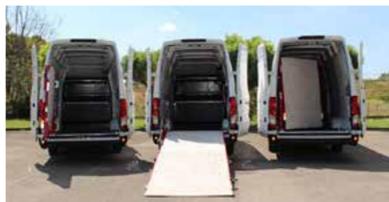
Shot-blasted non-slip aluminium surface
